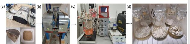
Sequential bioleaching of spent automotive catalytic converters (SACC): (a) SACC preparation, (b) magnetic separation, (c) indirect closed-loop leaching of base metals using biogenic H<sub>2</sub>SO<sub>4</sub> generated by bacteria, (d) direct bioleaching of platinum-group metals using a biogenic organic acid generated by a fungus.
